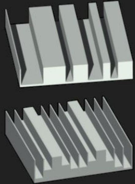
Figure XXX: Examples of maximum length sequence (MLS) acoustic diffuser pattern [left] and Quadratic-residue acoustic diffuser pattern [right]
