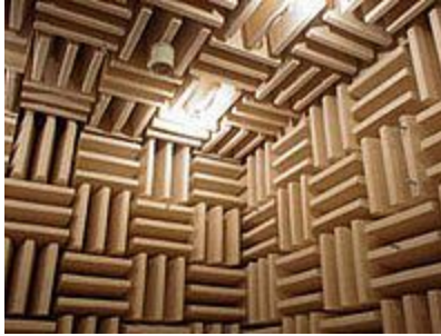
Figure 1.1. Example anechoic chamber (“Absorption (acoustics)”, 2017).
